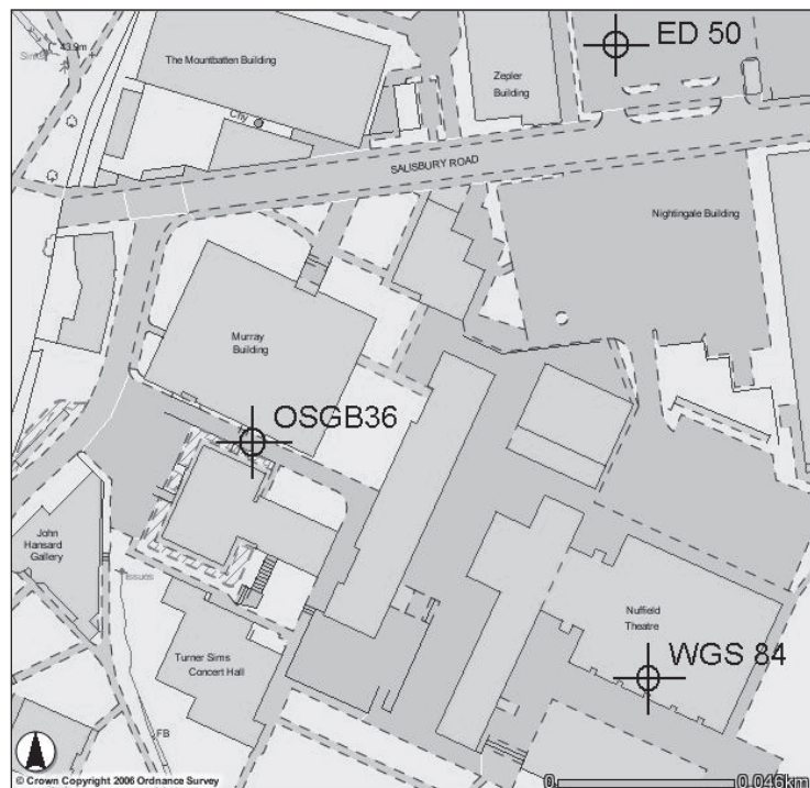
Figure 1: three points with the same latitude and longitude in three different coordinate systems. The map extract is 200 metres square.
