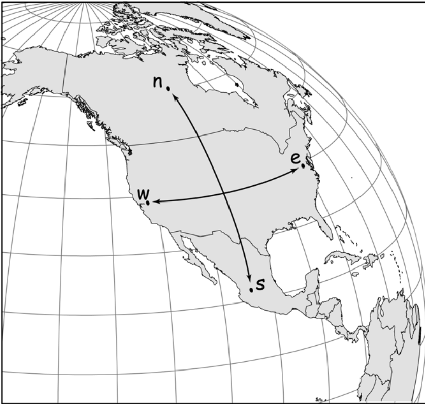
Figure 3-5: Two arcs illustrate the surface measurements and calculations used to estimate the semi-major and semi-minor axes, here for North America. The arc lengths may be measured by surface surveys, and the angles from astronomical observations, as illustrated in Figure 3-2 and Figure 3-3.
