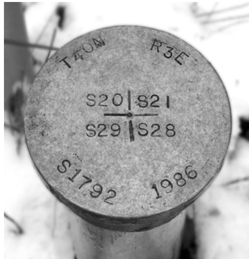
Figure 3-53: A PLSS corner that has been surveyed and marked with a monument. This monument shows the physical location of a section corner. These points are often used as control points for further spatial data development.
