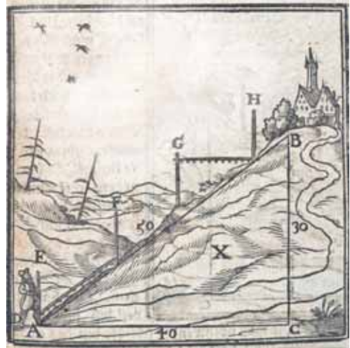
Figure 3-25: Early surveys used level bars placed on vertical posts, simple but effective technology.
