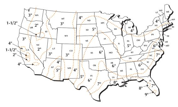
Use the above sketch in combination with the table of the variable rainfall rates below to determine the appropriate quantity and size of the roof drains required when you know:
