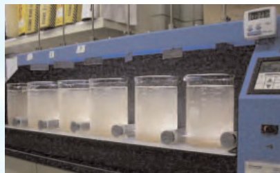
Testing at DEP water quality lab to determine alum dose
