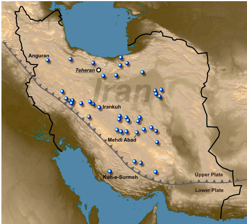
Fig. 7: Regional distribution of the non-sulphide zinc deposits. Most of these deposits are located on the upper (Iranian) plate. This plate has undergone strong uplift, exhumation, and erosion. (BORG ET AL. IN PREP.)
