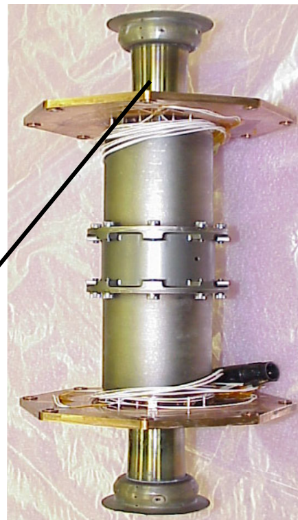
Paired converters with interconnect sleeve assembly
