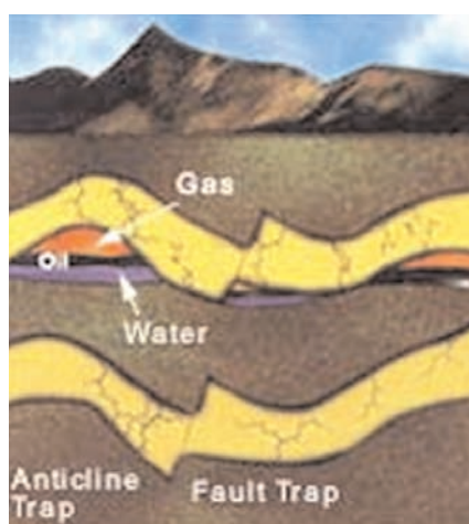
Figure 1 - Anticline and fault traps
