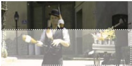
EMBEDDED ERROR OF 16 BYTES SET TO ZERO ON A JPEG IMAGE: THE RESULT IS A HALF IMAGE WITH A DRAMATIC LOSS IN COLOR QUALITY
