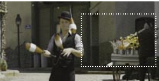
EMBEDDED ERROR OF 16 BYTES SET TO ZERO ON A JPEG 2000 IMAGE: THE RESULT IS A HALF IMAGE CORRUPTED WITH SOFT HIGH FREQUENCIES
