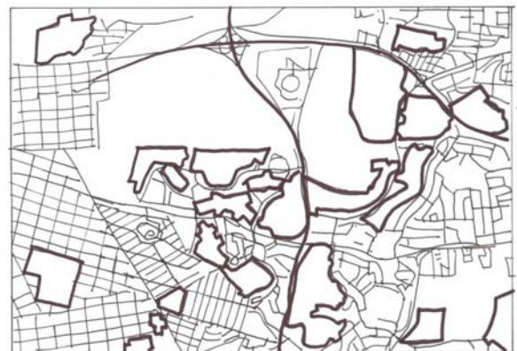
Figure 19: Transformed road network and urban form around Strubenkop, resulting in a gross urban fabric and a structure of super-blocks
