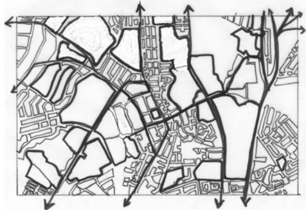
Figure 17: Transformed road network and urban form around Gallo Manor, resulting in a gross urban fabric and a structure of super-blocks
