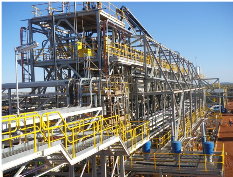
Figure 21. Flotation section at the Concentration plant at Mount Weld, Australia. Source: Lynas Corporation.
