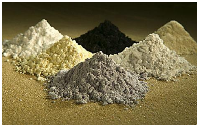
Figure 2. From top center, oxides of praseodymium, cerium, lanthanum, neodymium, samarium and gadolinium. Source: USDA.
