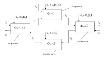
Fig. 12: System theory model of an electricitypowered heat pump
