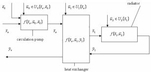
Fig. 15: System theory model of customer's heating/cooling system
