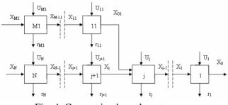
Fig. 4: Converging branch system
