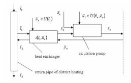
Fig. 11: In the case of obtaining the heat from the return pipe
