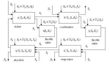
Fig. 13: System theory model of the absorption heat pump
