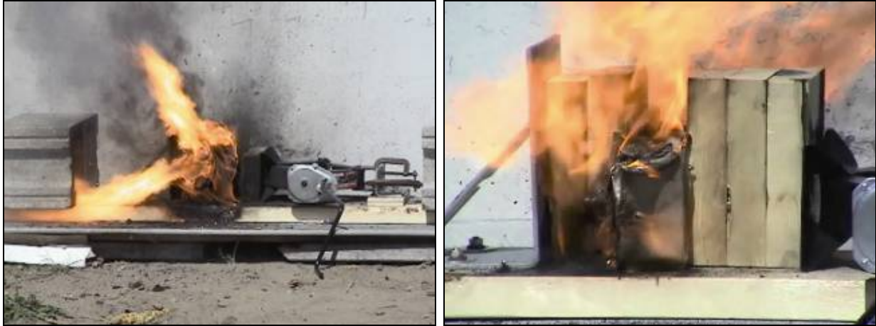
Figure 11: Comparison of the Flames Produced After Bullet Penetration of a BB-2590 Lithium-Ion Battery Containing Cylindrical Cells (left) and a BB-3590 Battery Containing Pouch Cells (the BB-2590 fire is far more violent).
