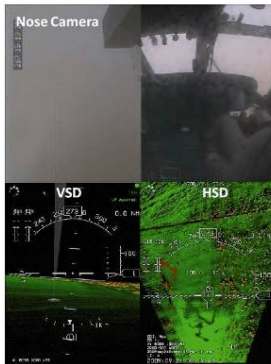
Figure 13: Helicopter Nose Camera View of Brownout Landing with No Visibility (top). Vertical (VSD) and Horizontal Situation Displays of LADAR Imagery with Symbology Overlaid.
