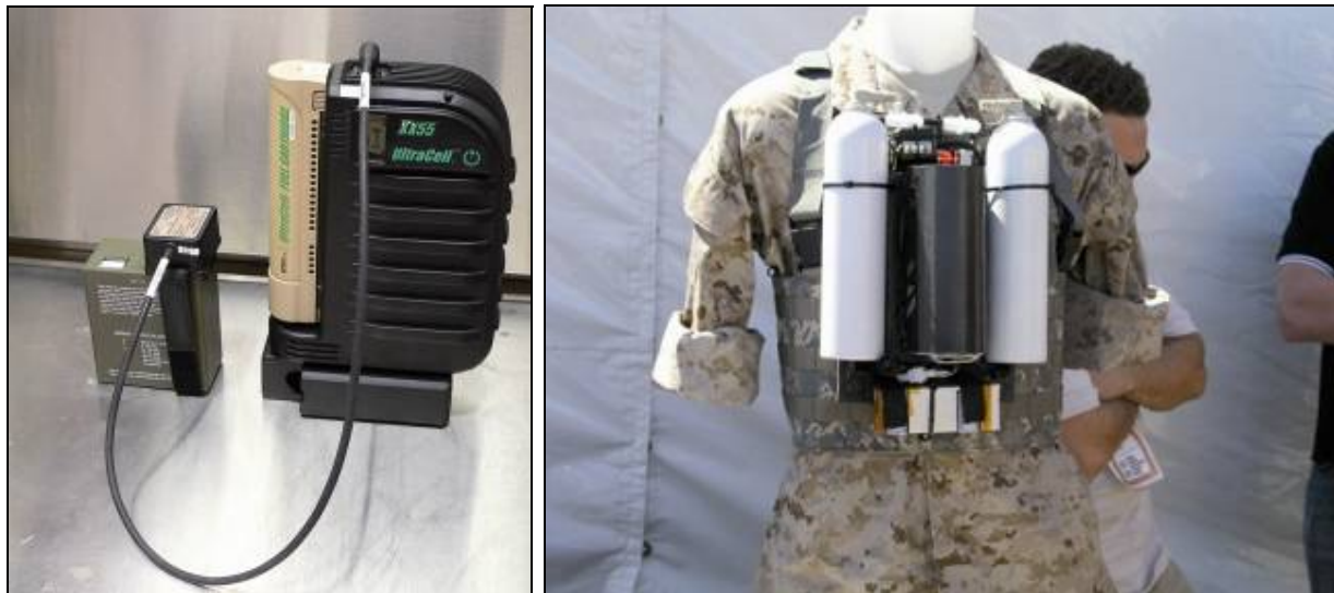
Figure 10: Left – 50 W Reformed-Methanol Fuel Cell Being Used to Recharge a BB-390 Battery (the beige portion of the fuel cell is the fuel canister); Right – Demonstration Solid Oxide Fuel Cell System Designed for 20 W Over 96 Hours.
