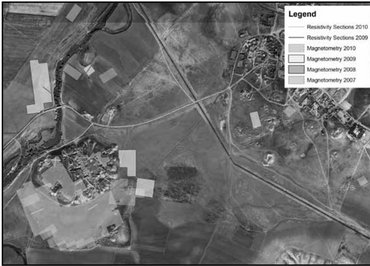
Fig. 1: Remote sensing activities on and around the Citadel Mound of Gordion, organized by year of exploration.
