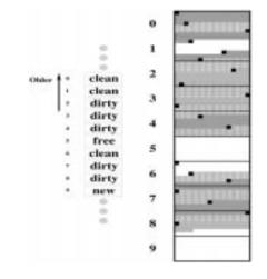
Figure 2: Compression Cache: Pages are compressed in the circular buffer, begun with header information, and described in a separate array that maps slots to physical page addresses and maintains current page state. The different patters refer to dirty, clean, and free compressed pages in memory.
