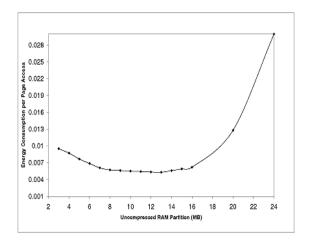
Figure 5: Energy consumption for various RAM partition configurations
