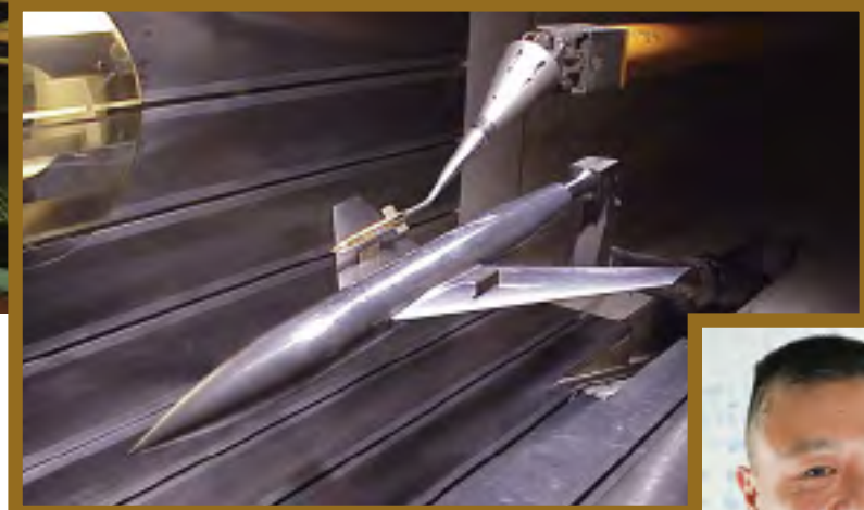
The release of a store off a South African Air Force Hawk is simulated in the image top left. Above: Two CSIR engineers prepare for the testing of a model aircraft in the CSIR medium-speed wind tunnel. Pictured in the inserted photograph is a store release validation, undertaken in the medium-speed wind tunnel at the CSIR, using generic parent and store models. Sean Tuling (right) of the CSIR says an aircraft's aerodynamics influences the trajectory of a weapon when it is released
