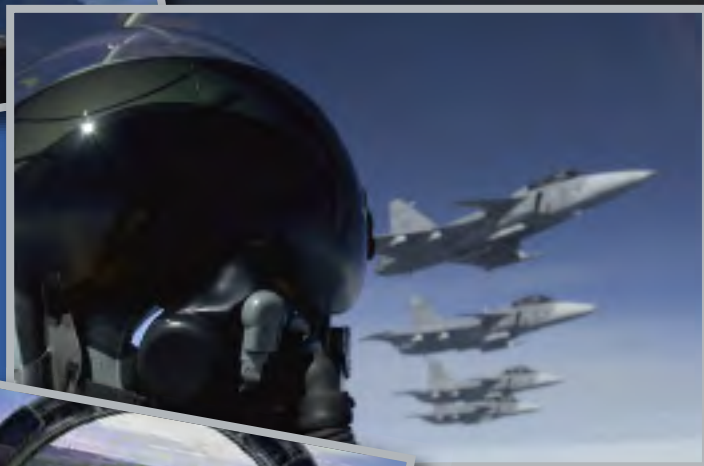
The Cobra helmet, as used in the SAAF's Gripens, can display critical data directly onto the visor and tracks where the pilot is looking. Displaying information on the pilot's visor means that the pilot does not have to continually glance down at the cockpit instrumentation while the head tracking allows aircraft sensors to be automatically directed towards targets of interest. Images copyright Gripen International Photographer: Katsuhiko Tokunago
