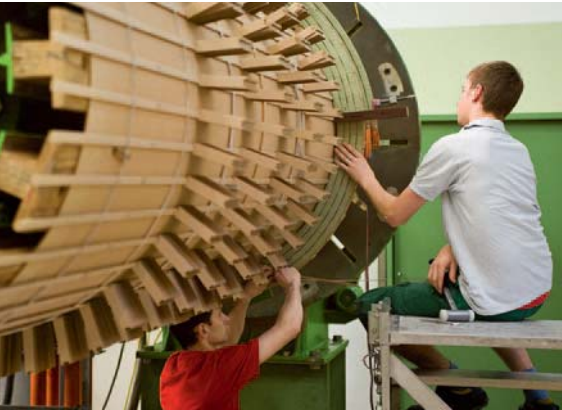
PLANT IN WEIZ. Specialists take many hours manufacturing the windings.
