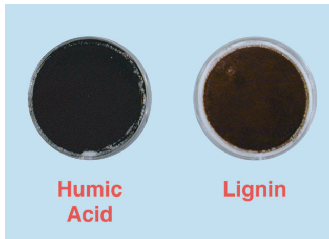
Fig. 2. Filters loaded with commercial samples of humic acid (Fluka 53680) and lignin (Aldrich 37,095-9).
