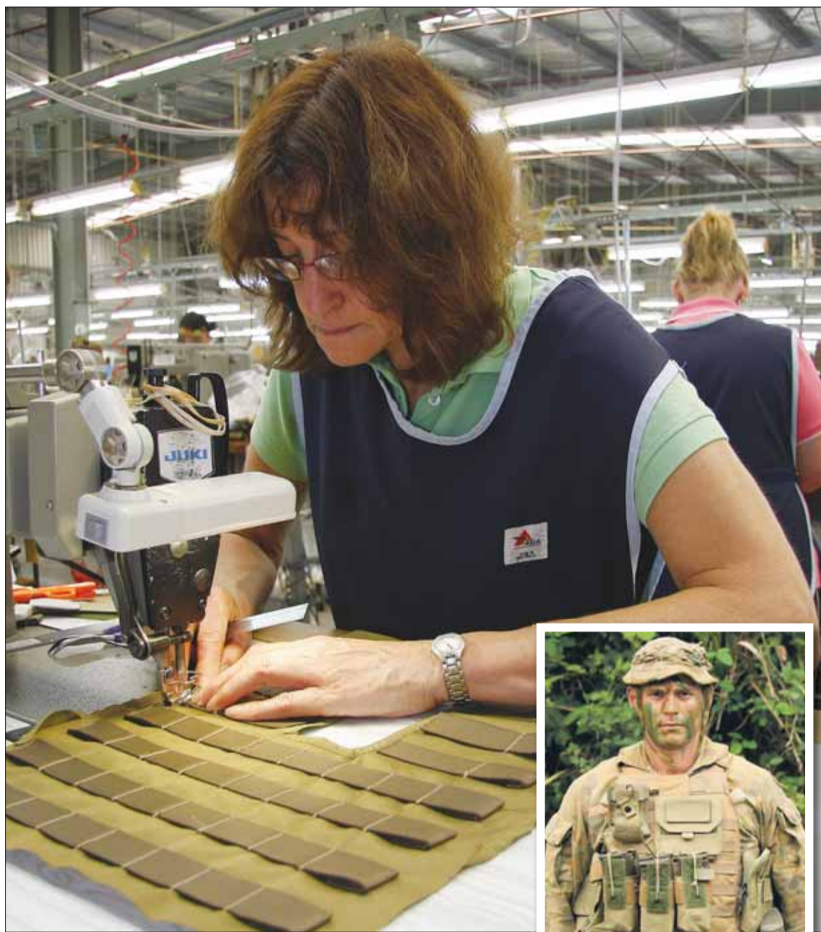
Fine tuning: Machinist Carolyn Lamshed attaches webbing tapes to the rear panel of the TBAS vest (above) and one of the new vests is modelled by a soldier (inset). Photo by Sgt Andrew Hetherington
