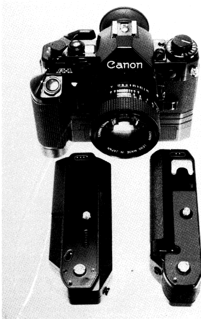
The Canon A-1 with motor drive and NiCad power pack mounted; below are the AA-battery power pack for the motor drive (left), and the smaller Canon winder for the A-1 and A-series cameras in general.
