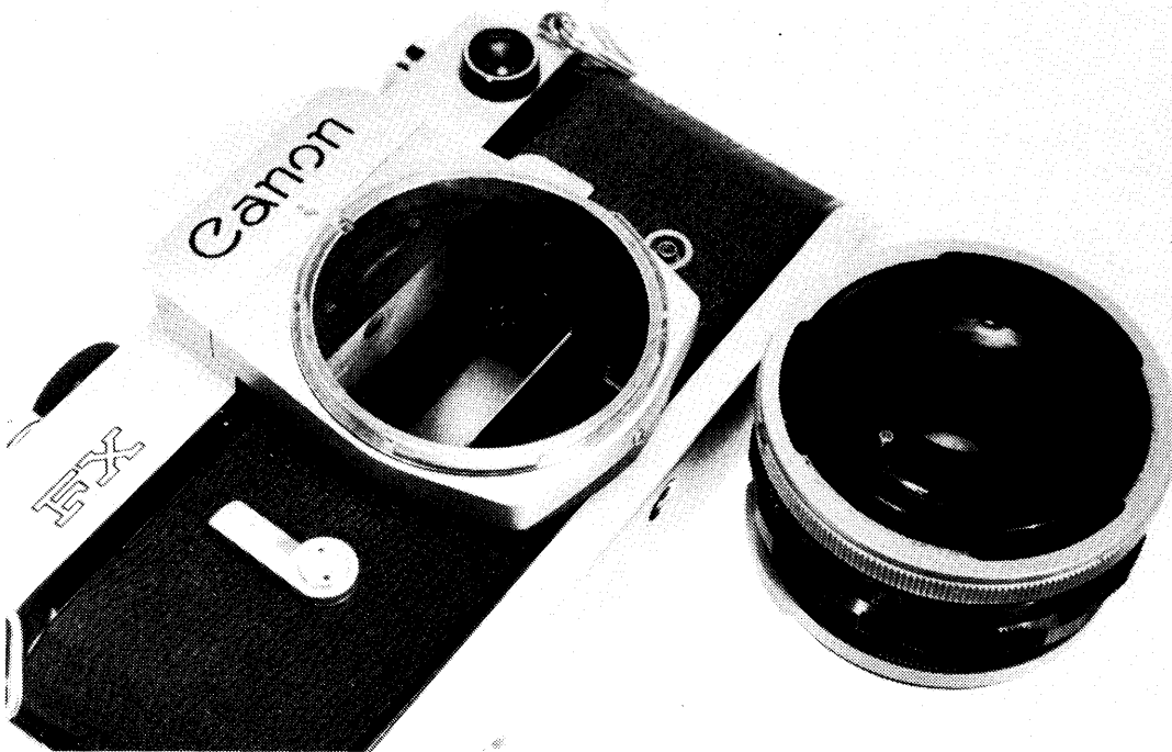
The FL lens and camera flanges, in which a single operating pin replaced the double set found on the original R-mount Canonflex lenses.
