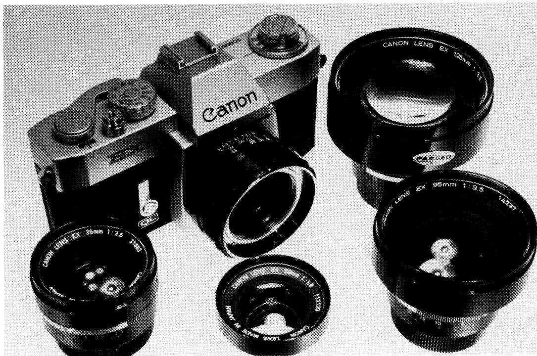
Here is the unusual Canon EX-EE with all its lenses: clockwise from top right they are the 125mm f/3.5, the 95mm f/3.5, the standard 50mm f/1.8, and the 35mm f/3.5. The camera is shown with naked lensmount into which each optic, which also fitted the later EX Auto, could be inserted. Each lens is marked "EX", just as was the Exakta lens shown in Chapter One, but obviously the two styles are not exchangeable.
