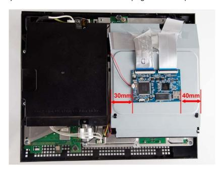
14. With a sharp knife or wire cutters remove part of the plastic case as shown
