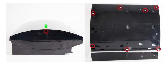
3. Remove the retaining screws and top cover from your  $\ensuremath{\mathsf{PS3}}$
