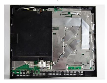
6. Connect the 3K3y power Y lead to the PS3 motherboard, ensure the double end of the Y lead is connected to the PS motherboard
