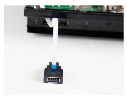
17. Plug the USB adapter into one of the PS3's USB sockets
