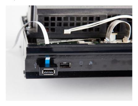
18. Connect the 3K3y 4 way FFC to the 3K3y PCB ZIF connector marked USB. The 4 way FFC should be routed tidily and may be secured with tape. Note, the blue plastic reinforcement of the 4 way FFC must be facing up.
