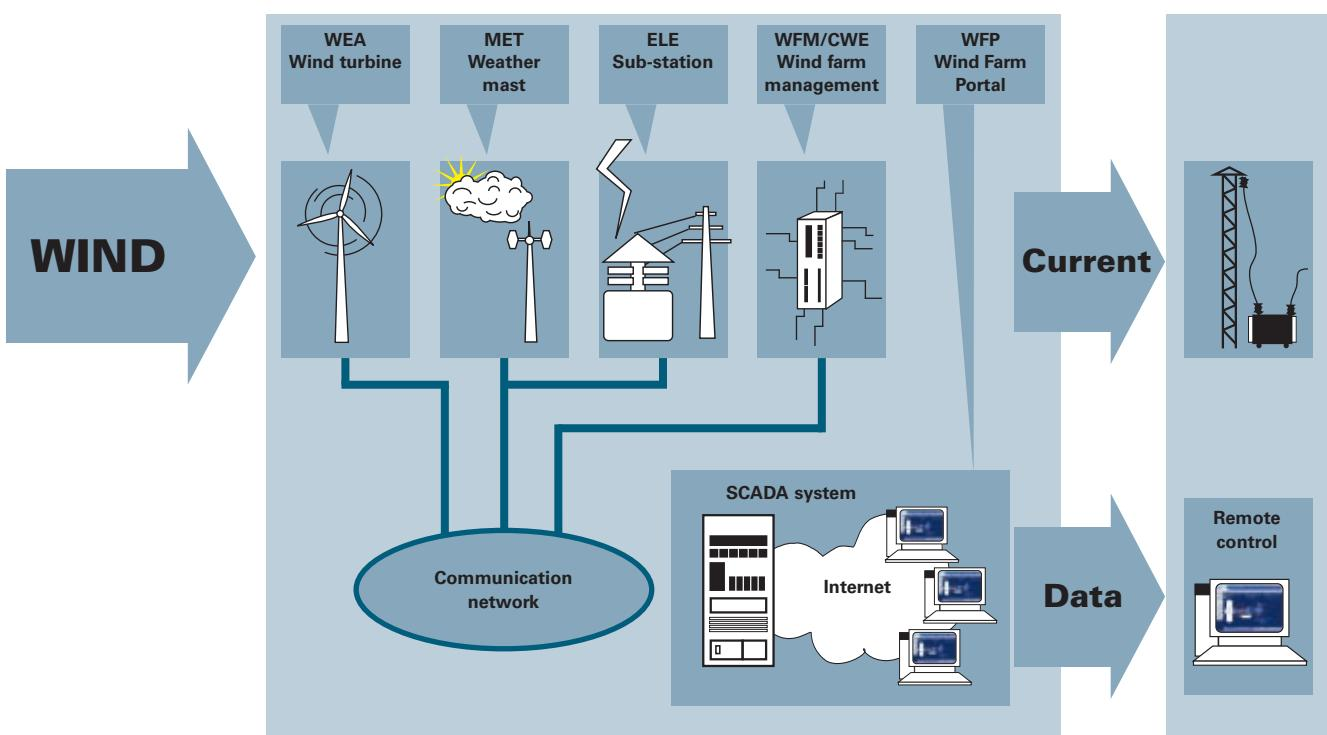
**The Nordex Control 2 Wind Farm Portal®** registers all the data concerning individual wind turbines, the meteorological and management systems, the sub-station as well as the complete wind park.
