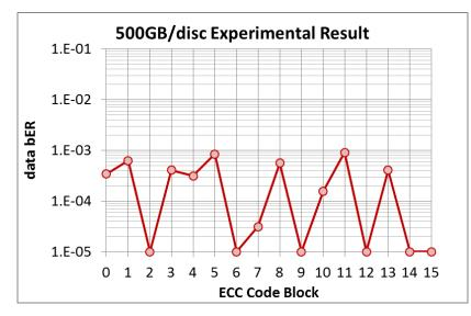
Figure 11. 2<sup>nd</sup>-generation AD recording/playback performance
