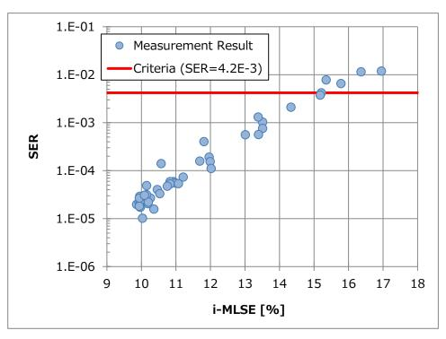
Figure 9. i-MLSE signal quality evaluation index and SER
