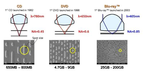
Figure 3. CD, DVD, Blu-ray Disc<sup>™</sup> playback spot and recording mark shapes
