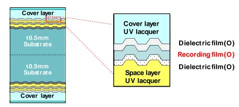
Figure 6. AD disc recording film
