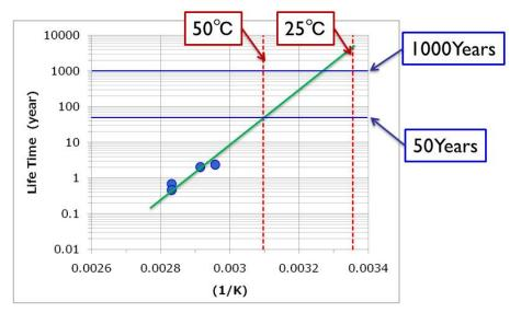
Figure 10. Long-term storage reliability in AD discs
