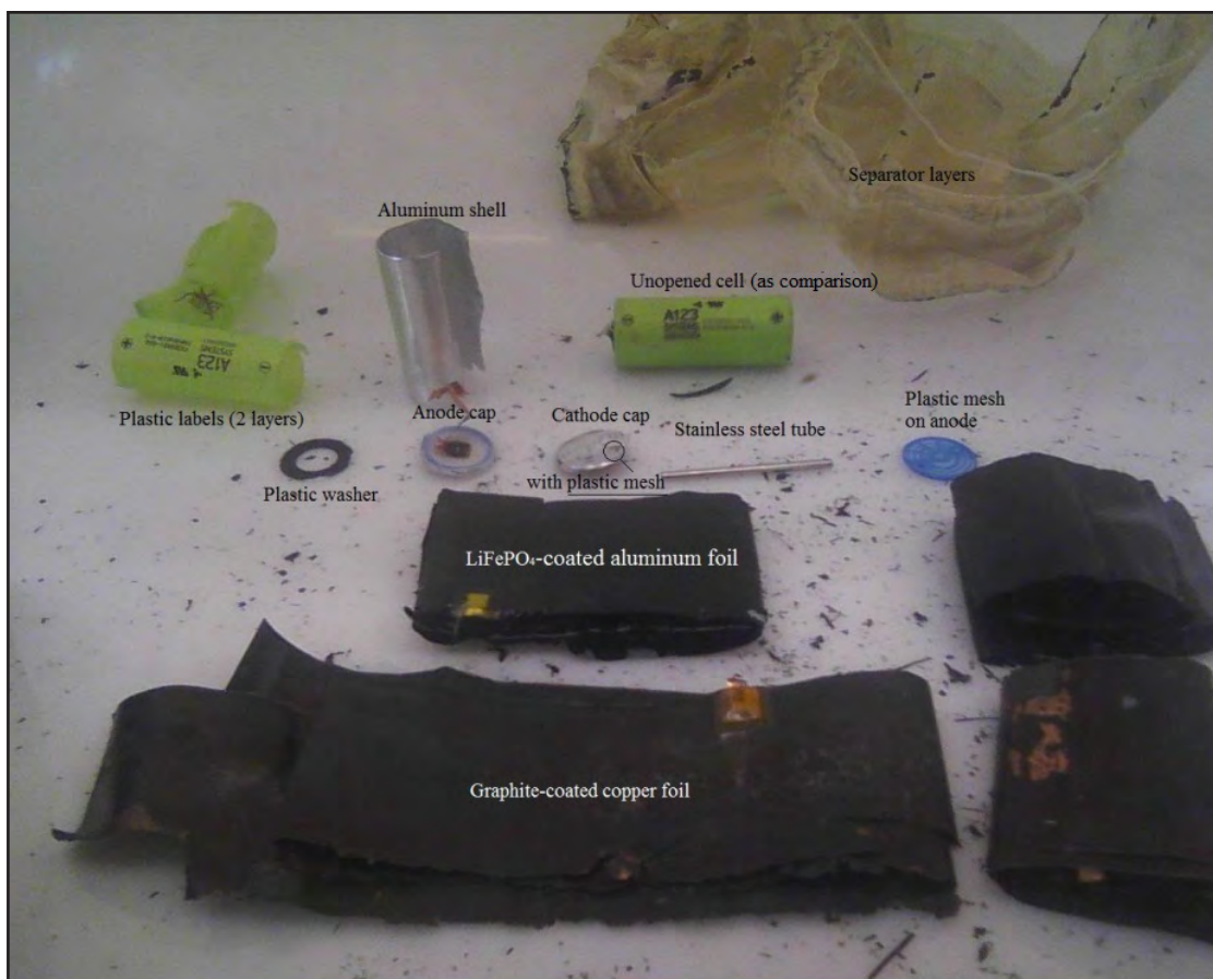
Figure 16. Layout of a Disassembled \text{LiFePO}_4 Cell with an Unopened Cell
