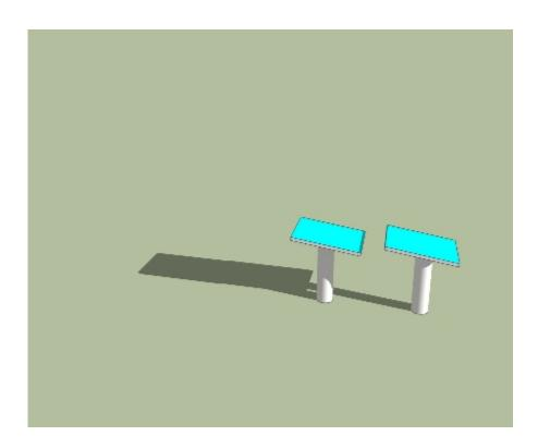
Low Sun Angle Single Axis System with Backtracking
