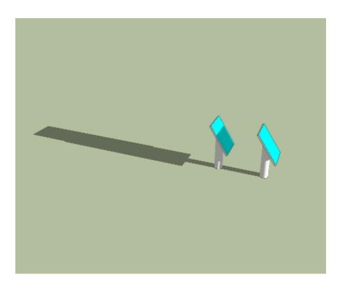
Low Sun Angle Single Axis System No Backtracking
