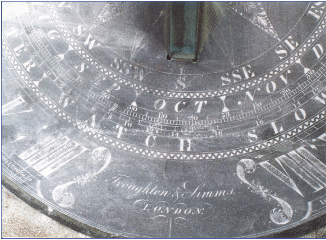
Fig. 10. A high-quality dial by Troughton & Simms, one of the last of the mathematical instrument makers producing dials. Talc has been used to highlight the engraving.
