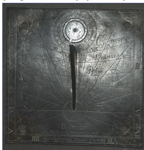
Fig. 3. A very simple Tudor dial almost without decoration and made with the use of punches. Note, in passing, the decorative shape of the gnomon – an area for further study.
