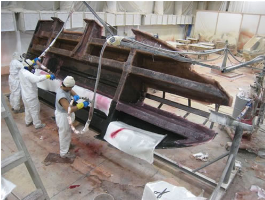
Figure 2. Hull Structural Grid System
