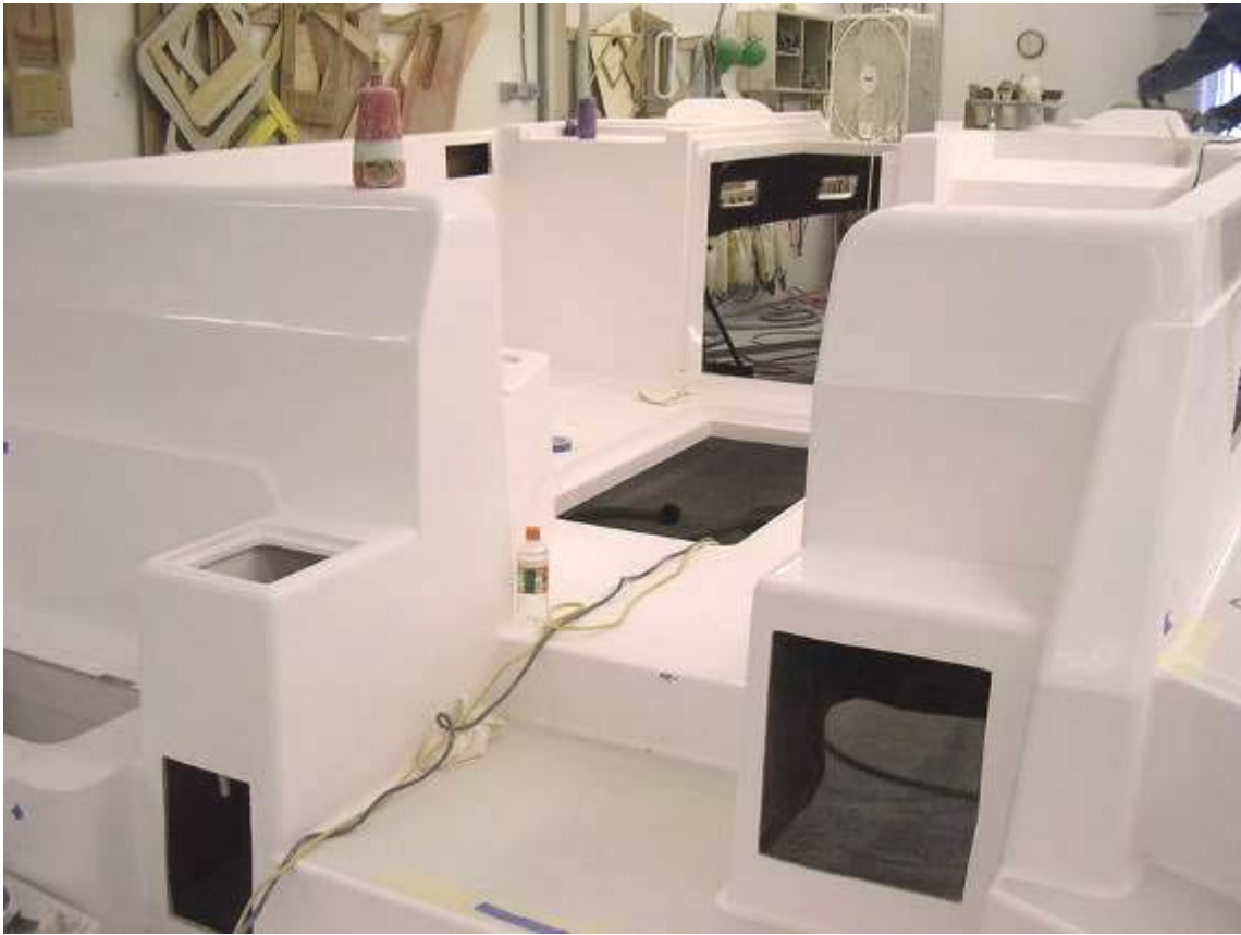
Figure 3. Complex Deck Part Built by Sabre Yachts
