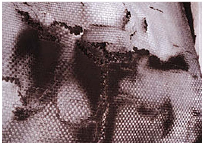
Figure 10. Composite Laminate after Structural Integrity Fire Test
