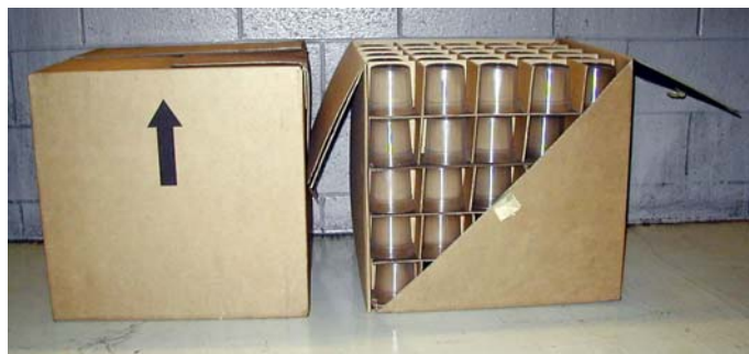
Figure 21. Prototypical Class A Commodity, 16 oz. polystyrene plastic jars in corrugated carton
