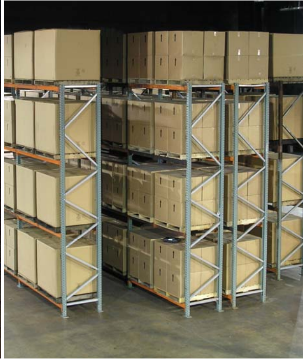
Figure 23. Example Fire Test Rack Storage Array
