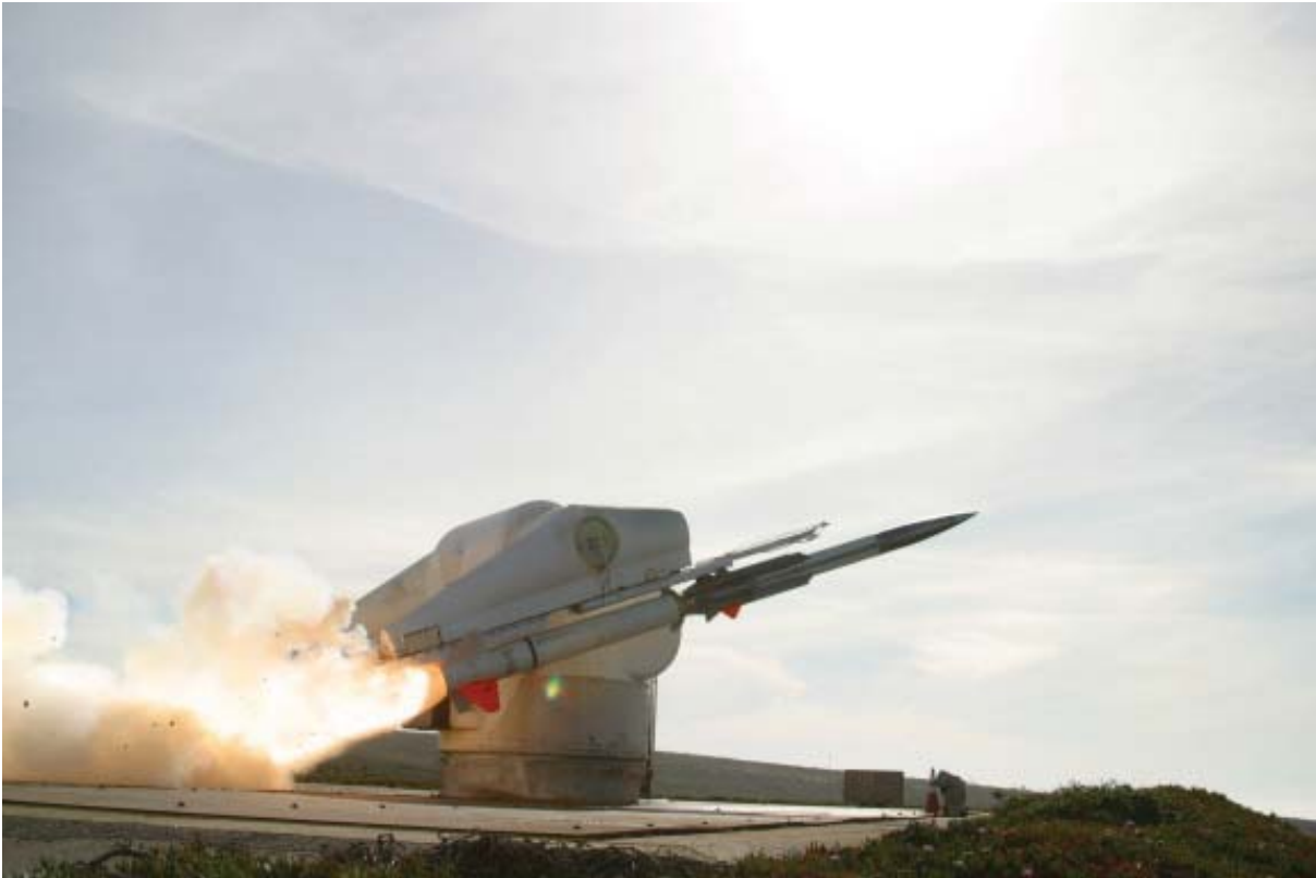
Figure 4. Coyote missile with booster and launcher at the Alpha Launch Complex on SNI (photograph by U.S. Navy).
