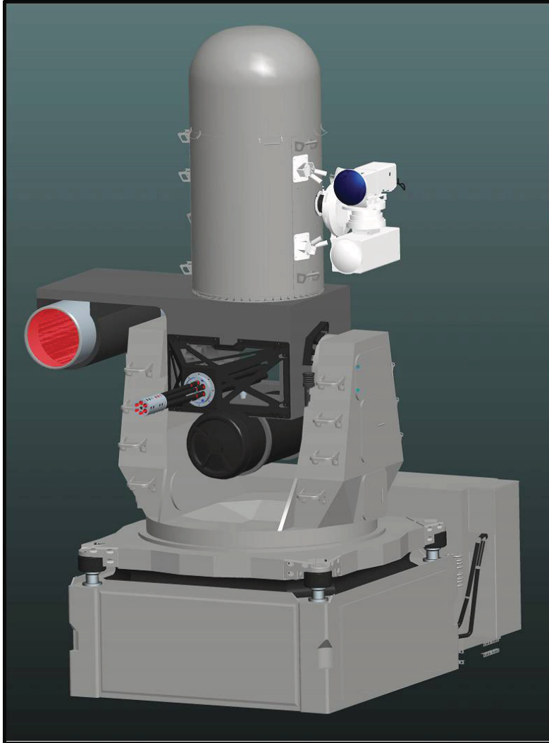
Figure C-2. Rendering of LaWS Integrated on CIWS Mount
