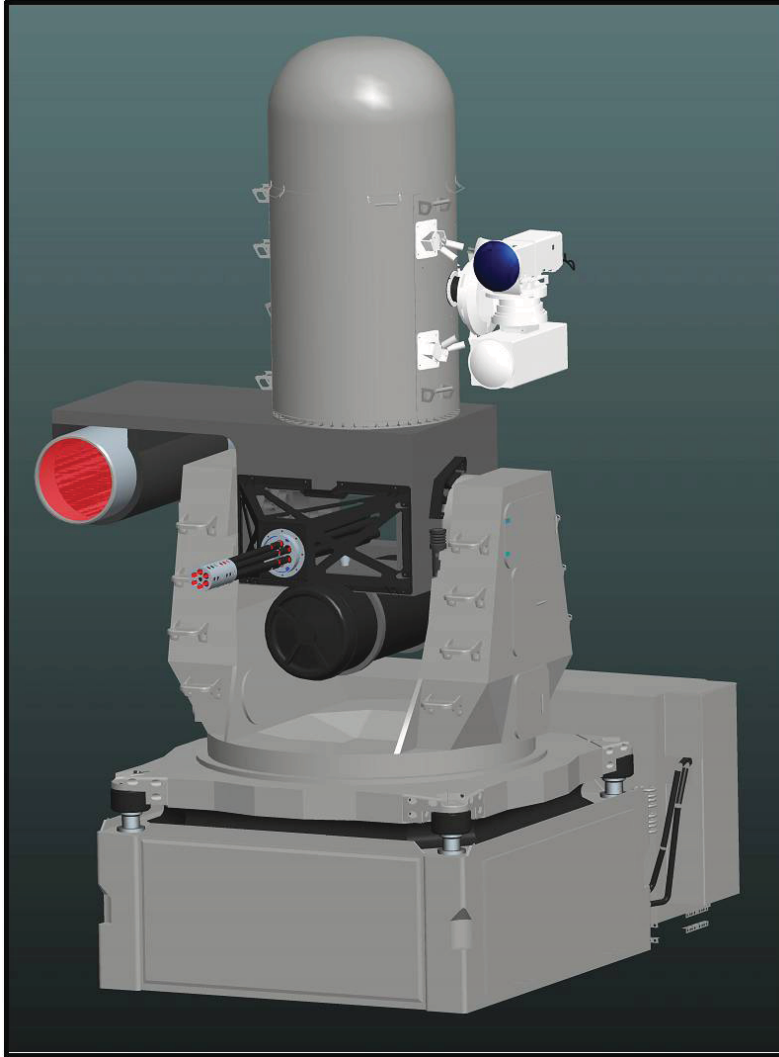
Figure C-2. Rendering of LaWS Integrated on CIWS Mount
