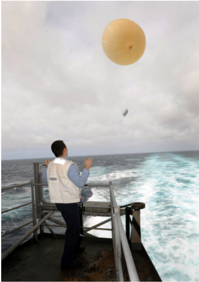
Figure 3-DOD10. Aerographer's Mate Airman Jonathan Salgado launches a weather balloon from the fantail of the aircraft carrier USS Theodore Roosevelt (CVN 71) to gather atmospheric data. (U.S. Navy Photo by Mass Communication Specialist Seaman Andrew Skipworth)
