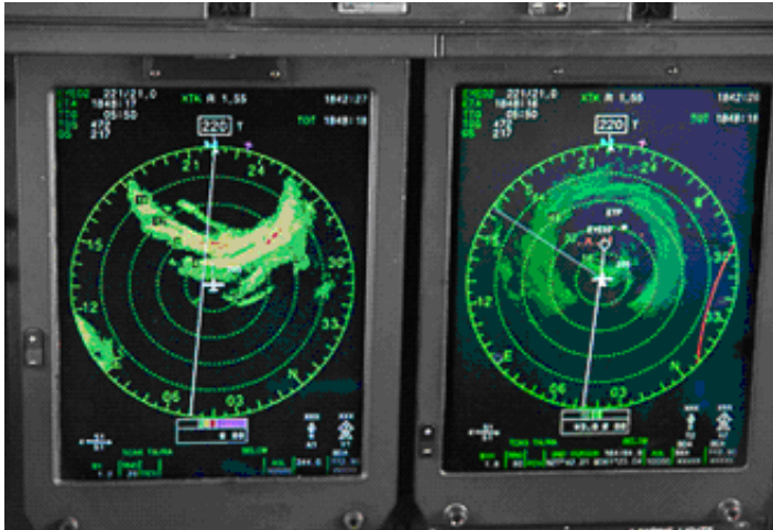
Figure 3-DOD-4. 53 WRS “Hurricane Hunter” WC-130J aircraft on-board radar (53 WRS Web site)
