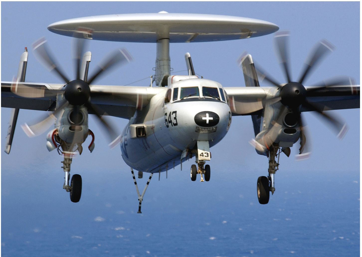
Figure 3-DOD-9. A Navy E-2C Hawkeye approached for an arrested landing on the flight deck of the aircraft carrier USS Harry S. Truman (CVN 75). The Hawkeye is the Navy's all-weather, carrier-based tactical battle management airborne early warning, command and control aircraft. (U.S. Navy photo)
