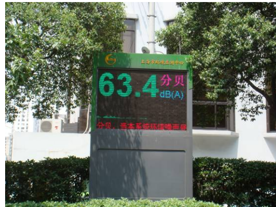
Figure 2-27: Noise-level Display Panel
