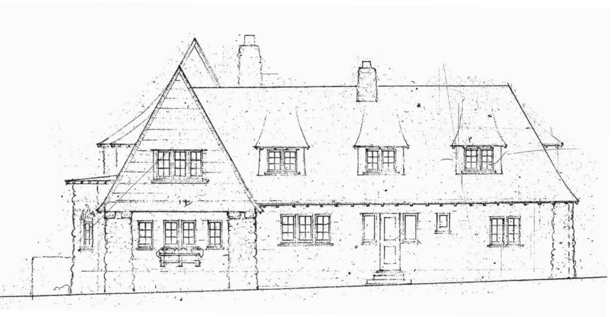
Figure 3.15: East Elevation of proposed clubhouse, March 1919. Note the stone terrace, stone pilaster corners and the swept dormer roofs. (eTIC)
