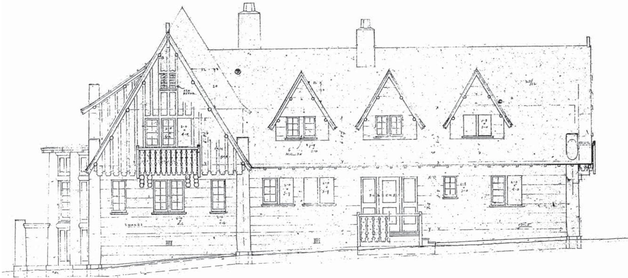
Figure 3.16: East Elevation of final design, March 1920. Note the change of stone piers to cedar log engaged columns, and the development of detail on the gable end. (eTIC)
