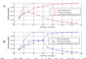
Figure 12. Blocking Probability Vs No Of Nodes For C=25 Using Heuristic Routing Algorithm A. Long Lightpaths B. Shorter Lightpaths.
