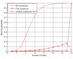
Figure 10. Blocking Probability Vs No of Nodes for C=25 And N=14
