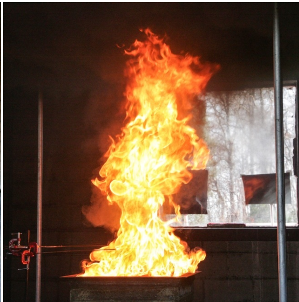
Fig 4: Fully Developed Pan Fire
