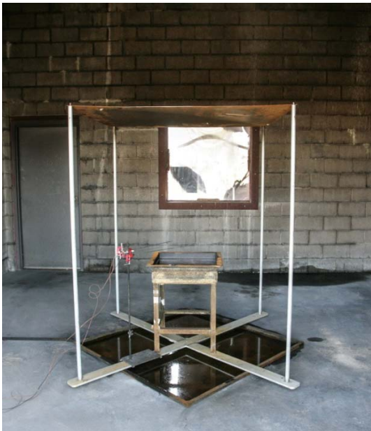
Fig. 3: Pan Fire Test Setup
