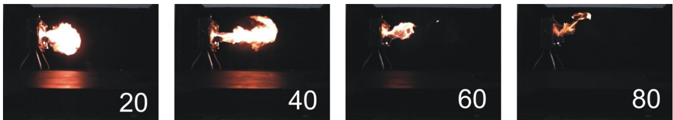
Fig. 1. Sequence of an exemplary deflagration, number indicates frame (210 fps)
