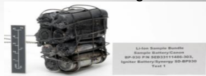
Test with Extinguisher
