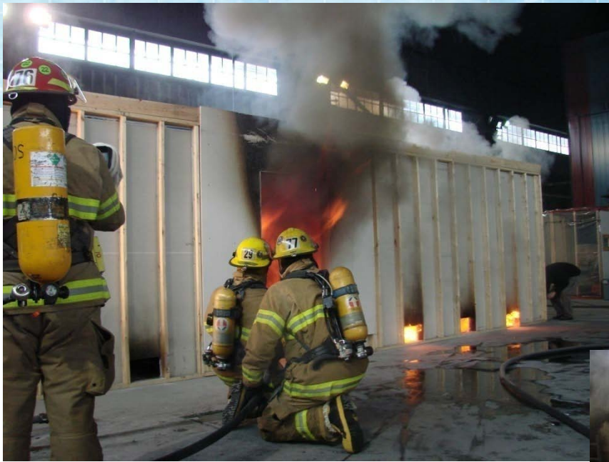
3 min after ignition (Flashover)
