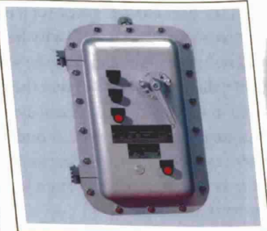
Exhibit 501.16 A magnetic motor starter for use in a Class I, Group D location. Note the number of securing bolts and the width of the flange. (Courtesy of O-Z/Gedney, a division of EGS Electrical Group)
