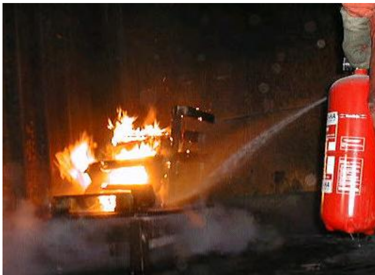
Figure 3. Class A pallet fire in Norwegian extinguisher tests [Jensen, 2006]
