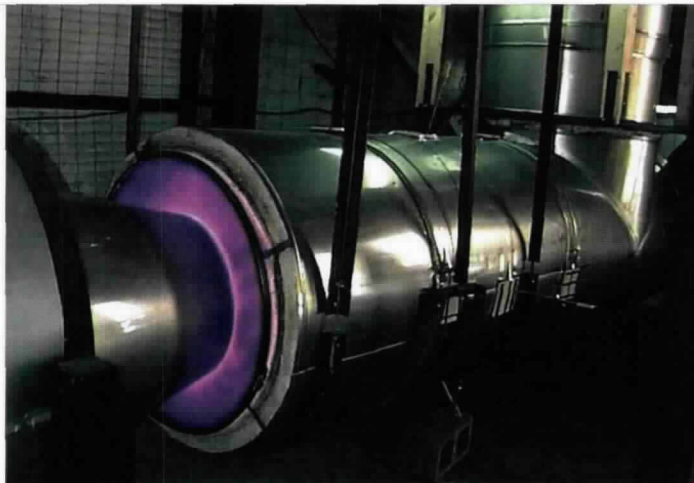
Factory-built grease duct undergoes extreme heat testing.
