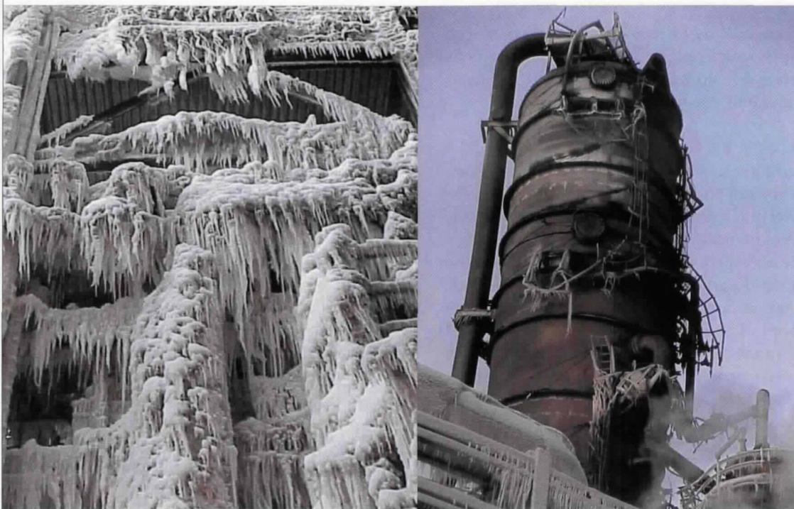
The fire at the Suncor facility required battling a blaze under the toughest of conditions. From left to right, frozen fractionator towers and the peak of the tower after extinguishment.
