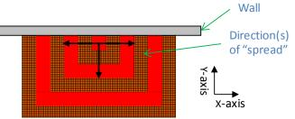
Figure 5 – Image Illustrating Lateral Fire Spread used in Fire Scenario 2.
