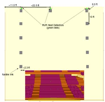
Figure 8 – RoR detector and fusible link placement (fire curtain release line) on the proscenium wall (elevation looking into auditorium through the proscenium opening) for the medium-sized theatre.
