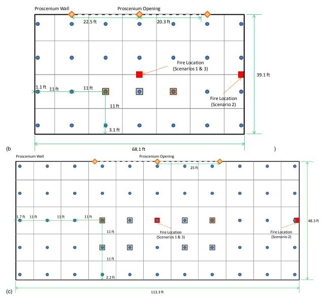
Figure 7 - Instrument layout shown in reflected-ceiling plan in the (a) small, (b) medium, and (c) large theatre models ( $\bullet$  - sprinkler;  $\diamond$  - heat detector;  $\Box$  - smoke vent fusible link;  $\blacksquare$  - fire locations).
