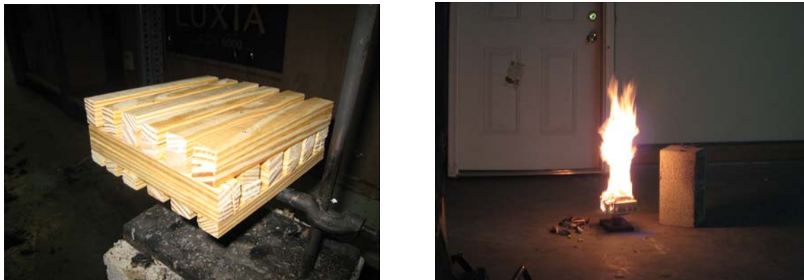
Figure 14: UL 268 Wood Crib Fire Configuration & Fire
