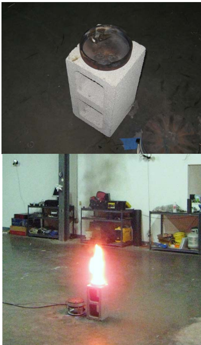
Figure 8: UL 268 Flammable Liquids Fire
