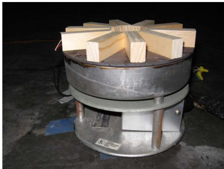
Figure 11: Elevation View of UL 268 Smoldering Wood Configuration
