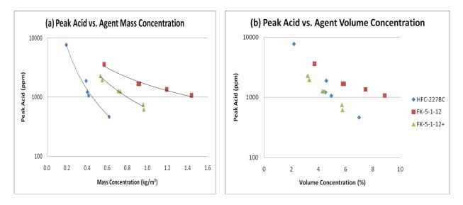
Figure 6. (U) Peak Acid levels for 'HFC-227BC,' 'FK-5-1-12+' and 'FK-5-1-12' (ref. 13b) versus Agent a) Mass and b) Volume Concentrations. The solid lines in (a) are power curve fits. Note: Although the peak acid levels for 'HFC-227BC' and 'FK-5-1-12+' are similar, the integrated levels used in casualty assessments were very different: none of the FK-5-1-12-based
