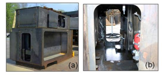
Figure 1. (U) Exploratory Test Box a) Exterior and b) Interior.
