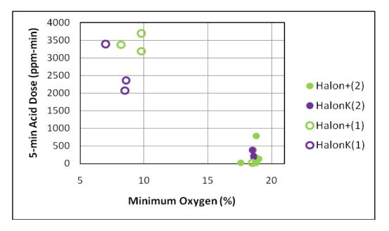
Figure 4. (U) Five-Minute Acid Dose versus Minimum Oxygen Level for Halon with Sodiumand Potassium-Bicarbonate Dry Chemicals (ref. 13e).
