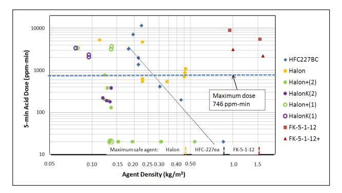
Figure 3. (U) Average Acid Dose Integrated over 5-Minutes versus Agent Density (ref. 13d,e). The solid line is a 'best fit' trend using a Power Series based on the 'HFC-227BC' data.
