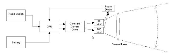
Figure 3 Emitter Unit Physical Architecture
