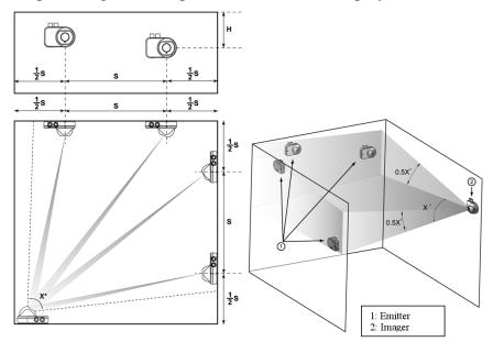
Figure 2 Multi-Emitter area OSID layout
