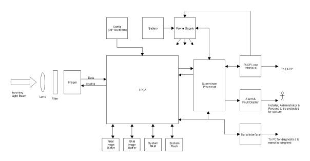
Figure 4 Imaging Unit Physical Architecture
