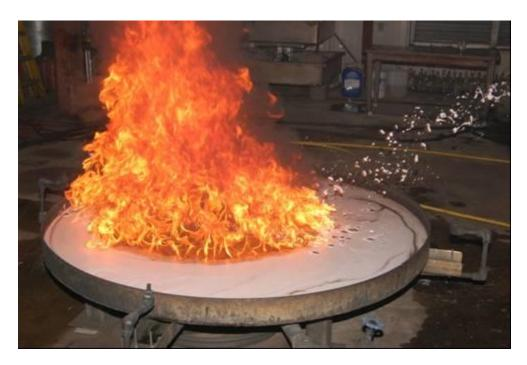
Figure 3. End of burn back test with JP-5. Unlike the gasoline test, the fire is confined to a well-defined foam-free area of the fuel surface. The foam-covered region does not have flames isolated from the main fire.
