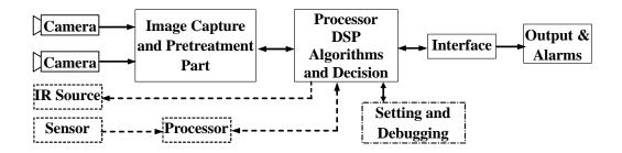
Figure 2. Schematic of the AlarmEye VID detector
