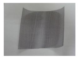
Figure 21. A metal mesh for light obstruction
