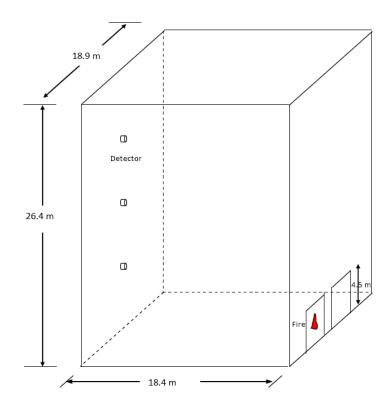
Figure 1. Schematic of test atrium, detector and fire locations
