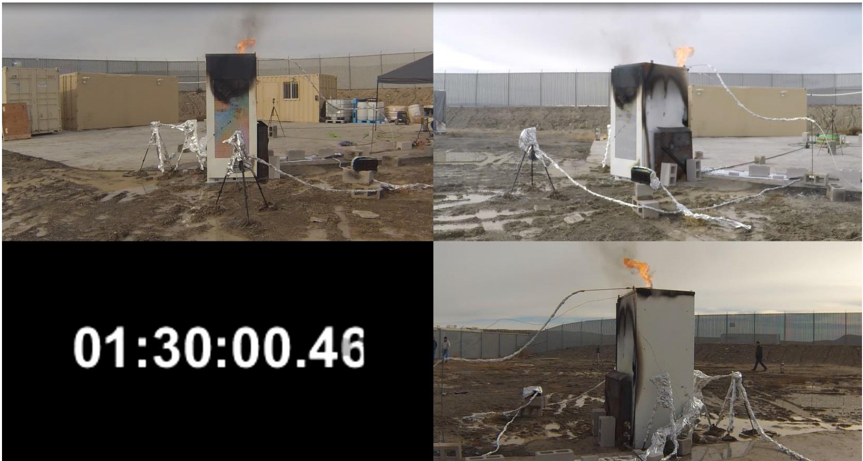
Figure 23 External test screenshot: test time = 1 hour 30 minutes, flames at front door and exhaust vent intermittently decreasing in intensity
