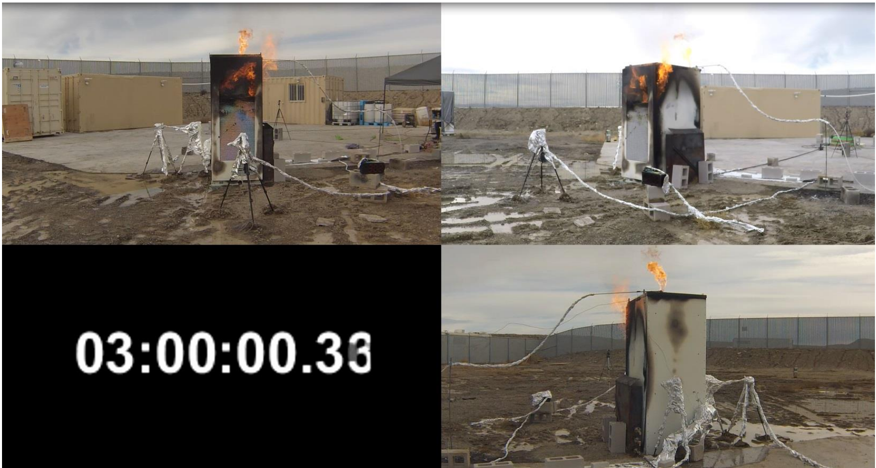
Figure 26 External test screenshot: test time = 3 hours, fire inside the Powerpack subsiding
