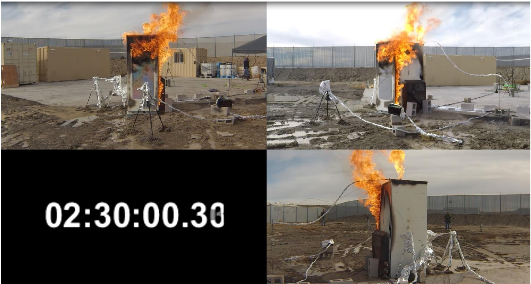
Figure 25 External test screenshot: test time = 2 hours 30 minutes, fire inside the Powerpack intensifying
