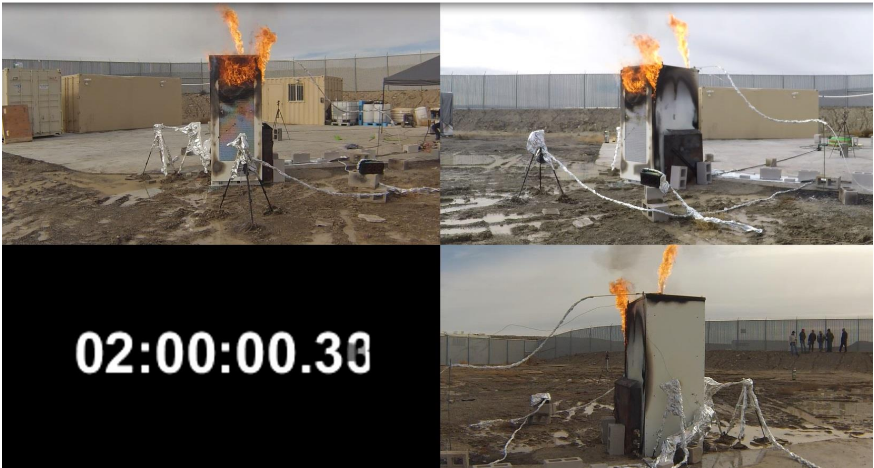
Figure 24 External test screenshot: test time = 2 hours, fire inside the Powerpack intensifying
