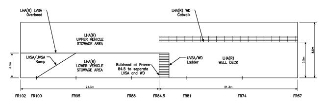
Fig. 1-ex-USS SHADWELL test area, section view
