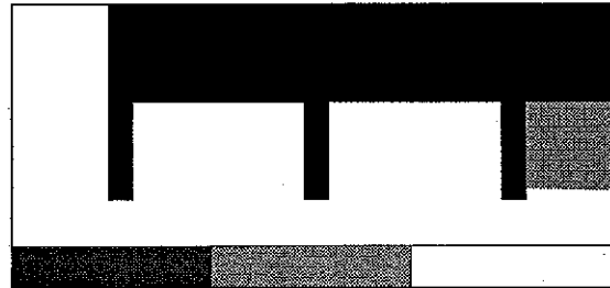
Figure 22: Shaded contour plot of heat detector (RTI = 300) response volumes for various beam depths: 0.0 m (0 in), 0.10 m (4 in), 0.20 m (8 in), 0.30 m (12 in), 0.61 m (24 in) with 3.35 m (11 ft) ceiling height, 1.22 m (4 ft) beam spacing and medium fire. Dark and light grey denotes where a sensor activates before the fire reaches 100 kW and 1.0 MW respectively. White denotes where the sensor would not activate. Activation criteria: when the link temperature rises to 57°C (135°F).
